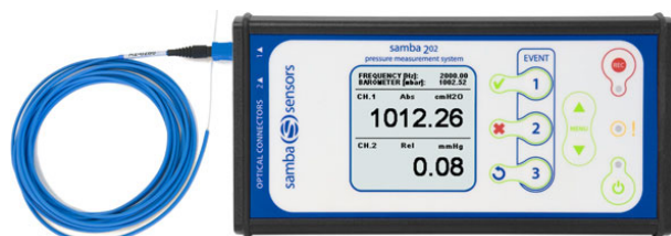
Control Unit with TSD170 series transducer
