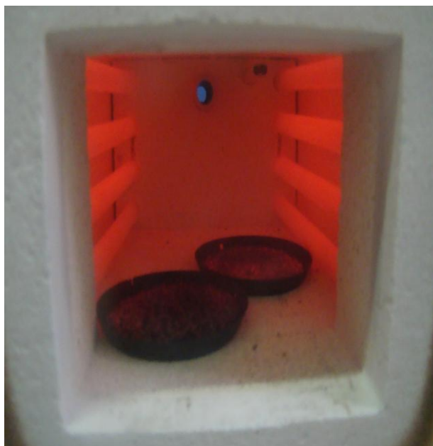
Fig. 3. Calcination stove to determine the ash content
