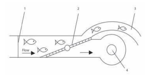
**Fig. 5.3.2.** Revolving screens are installed in a raceway – 1, screens – 2 are attached onto a swivel joint which enables turning over of the screens and rinses them with flowing water, the fish are guided by the screens to the bypass – 3, away from the SHPS turbine – 4 (scheme: P. Dvořák).
