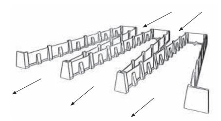
**Fig. 5.2.2.** Possible modification of a weir dam – elongation of the weir top with increased aeration (adapted from Adámek et al., 2010).
