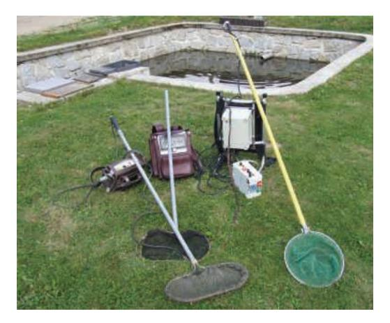
**Fig. 6.1.1.** Battery electrofishing devices of Czech and foreign production (left LENA, SEN – Bednář company, right IG200 – Kronawitter company) (photo: J. Turek).
