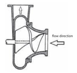
Fig. 5.3.12. Scheme of a fish pump (scheme: Clay, 1995).
