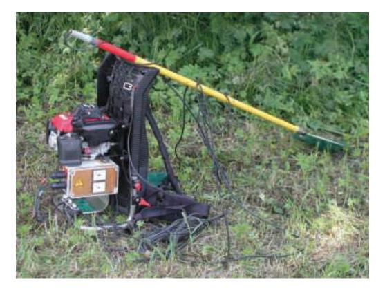
**Fig. 6.1.2.** Backpack engine electrofishing device produced by EFKO (Germany) with accessories (photo: J. Turek).
