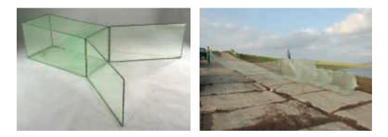
**Fig. 6.2.10.** The so-called Klíčavská fish pot with a solid metal frame (left, photo: P. Pokorný) and a photo of the stretched Římov pre-chamber fyke nets (Kubečka, 1992) with an antechamber of 1.5 x 1.5 m, with a chamber diameter of 0.9 m and a mesh size of 20 mm (right, photo: FISHECU).
