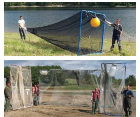
**Fig. 6.2.6.** Frame ichthyoplanktonic trawl used for catches of the earliest stages of fry in open waters of dam reservoirs (above, photo: P. Pokorný) and fry trawls used for catching juvenile fry later in the season (below, photo: FISHECU).
