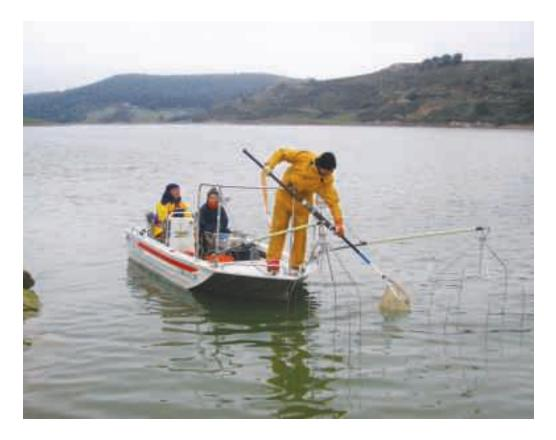
**Fig. 6.1.9.** Catches of older and adult fish are carried out by electrofishing with two anodes fixed before boats and equipped with steel cables, which are immersed in the water during catching (photo: M. Kratochvíl).
