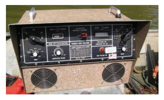
**Fig. 6.1.6.** A stand-alone power unit with options of setting parameters of the type of electrical current, settings of voltage, frequency, working cycle, etc. (Smith-Root, USA) (photo: M. Kratochvíl).
