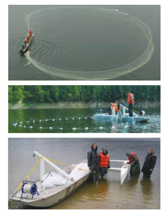
**Fig. 6.2.5.** Set adult purse seine (above), putting the net into the boat during working with purse seine (middle) and a boat with special modifications for handling purse seine used by the Hydrobiological Institute of the AS CR, v.v.i. – patent no. 302159 (below, photo: FISHECU).
