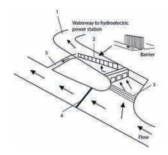
**Fig. 5.3.5.** Installation of the Louvre barrier into the raceway for the SHPS. Water is flowing through the raceway – 1 into the SHPS, fish are guided by the barrier – 2 back to the main stream under the weir – 4. Coarse impurities and water debris are caught by pre-screens – 3 (scheme: P. Dvořák).
