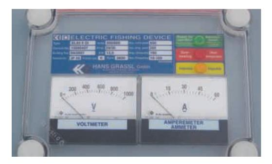
**Fig. 6.1.7.** Detailed view of the voltmeter and ammeter to measure the output voltage and current of the electrofisher (Hans Grassl, Germany) (photo: M. Kratochvíl).
