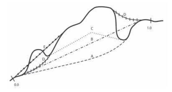
**Fig. 5.1.7.** Possible alterations to longitudinal geometry of a stream (according to Zelinka and Kubíček, 1985, adapted from Adámek et al., 2010). Note: A–E represent various options of solution (see the text).
