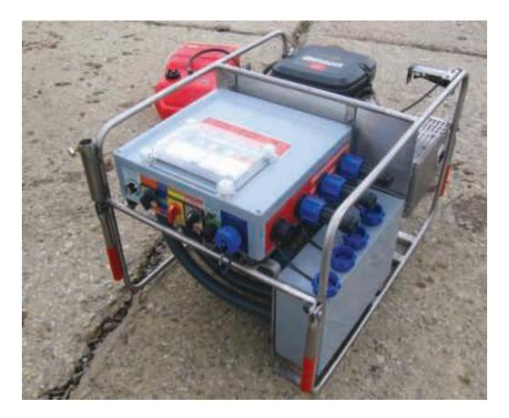
**Fig. 6.1.5.** An electrofisher commonly used for catching fish from boats in European running and lentic waters. The equipment also includes a power unit with outputs for connecting electrodes and an auxiliary fuel tank (Hans Grassl, Germany) (photo: M. Kratochvíl).
