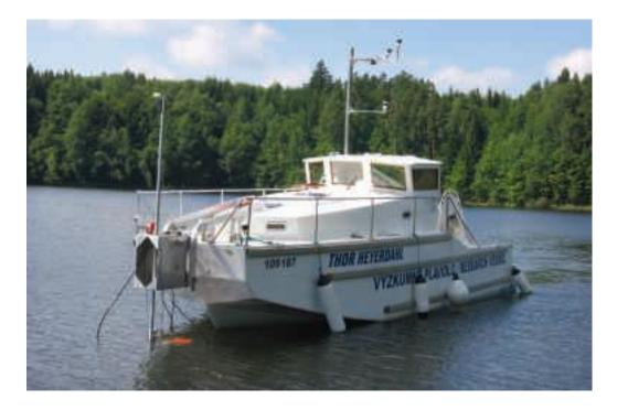
Fig. 4.2.1. Transducers in the fore part of the research vessel exploring the reservoir (photo: FISHECU archive).
