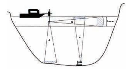
**Fig. 4.2.4.** Diagram of basic echo sounder surveys – vertical (A), horizontal (B) and reverse vertical (so-called up-looking) (C). In each case, ultrasound samples the volume of a conical shape. There is usually a short so-called dead zone in the vicinity of the transducer, the bottom and water level, where the record cannot be used for fish detection (hatched areas in the beams).
