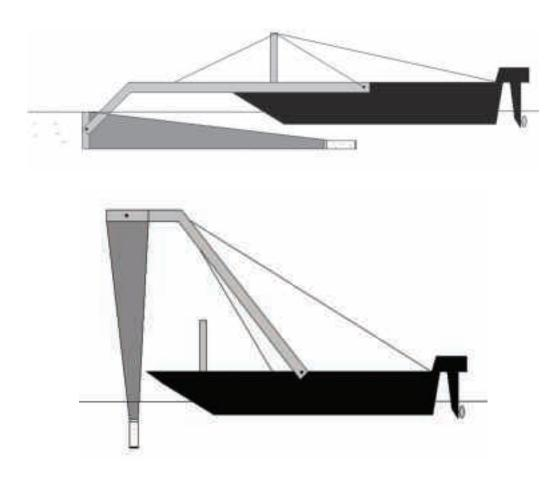
**Fig. 6.2.8.** Sketch of a net pushed in front of a vessel during sampling (top) and positions of the push net after sampling completion before emptying the catch (below, according to Herzig et al., 1994).
