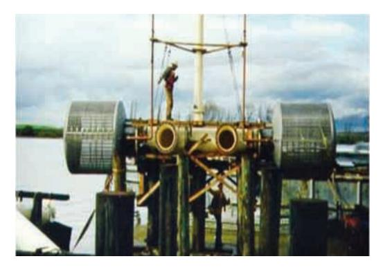
**Fig. 5.3.4.** Cylindrical barrels made of trapezoidal bars installed as a protective filter on piping taking off technological water (photo taken from http://www.bdiscreens.com/fishdiversion.htm used with the approval of Industrial Screen Products, Inc., P.O. Box 366, Placerville, CA 95667 USA).
