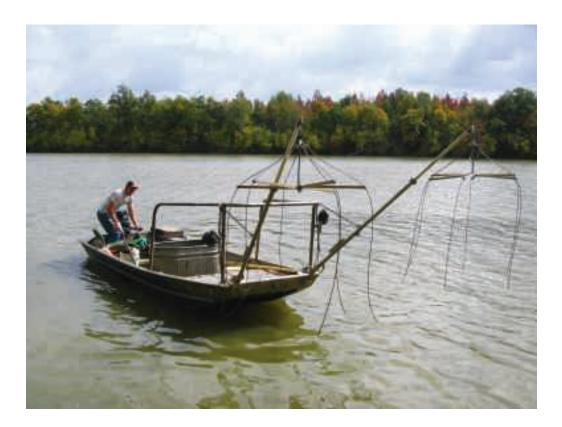
**Fig. 6.1.4.** An electrofishing boat with a safety railing and a system of two anodes placed obliquely in front of the vessel's hull (Smith-Root, USA) (photo: M. Kratochvíl).
