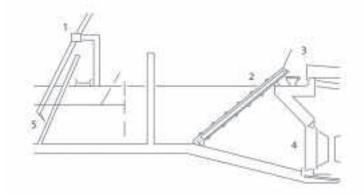
**Fig. 5.3.7.** Scheme of installation of the barrier in the form of a rotating mesh for derivative SHPS in Hadamar, Germany. Technological water from the raceway (5) flows through rough screens (1) onto rotating screens (2) that carries fish and minor impurities into the bypass (3). Water is subsequently taken off by the SHPS (4) (scheme: P. Dvořák).
