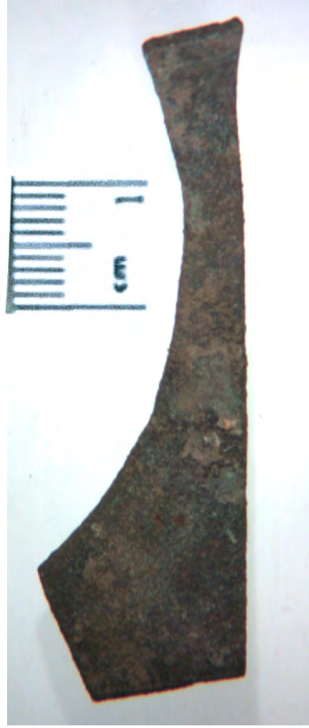
Fig.13 Specimen #14 annealed (a) but with ghost-like striations (b) due to deformation adjacent to cut edge. Also see corrosion spots (c) near cut edge with re-deposited copper.
