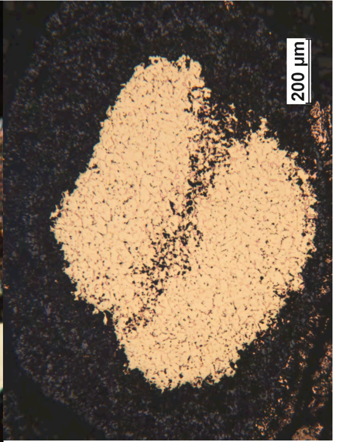
Fig. 17 Specimen #10 Folded assembly of brass and leaded bronze with included copper wire
