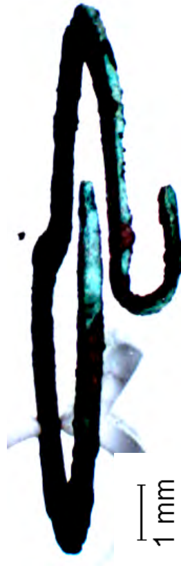
Fig.4. Specimen #1 In-plane (1L) showing deformation lines, and transverse (1T)
