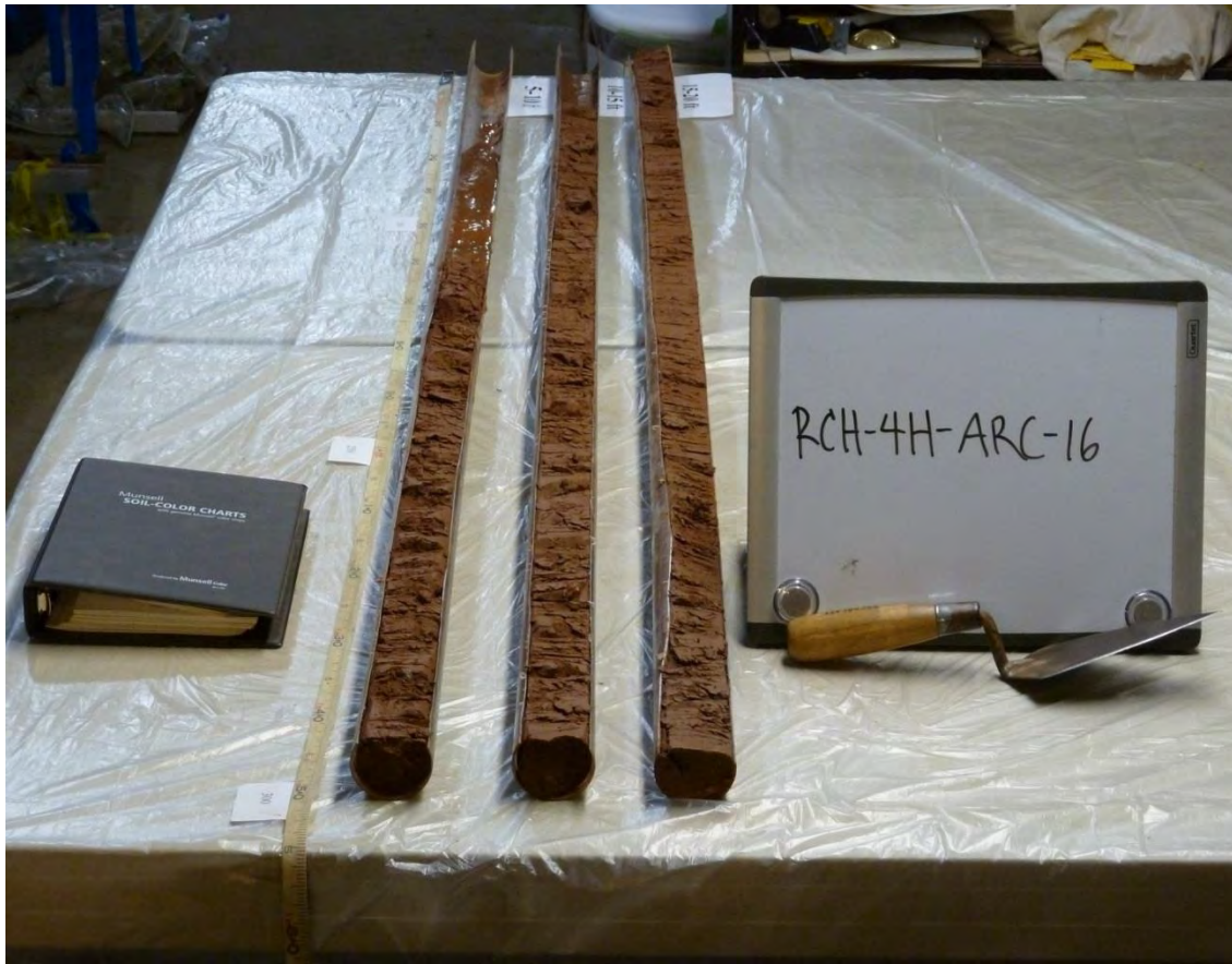
Figure 8: Split core prepared for documentation and sampling under laboratory conditions.
