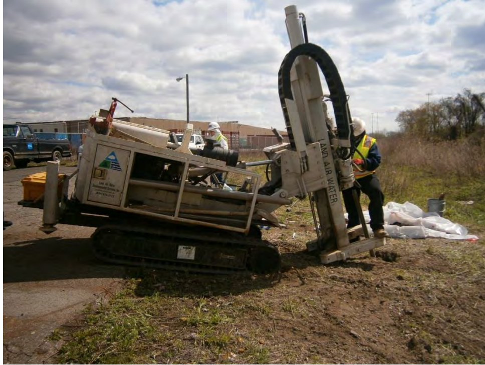
Figure 6: Field collection of cores.
