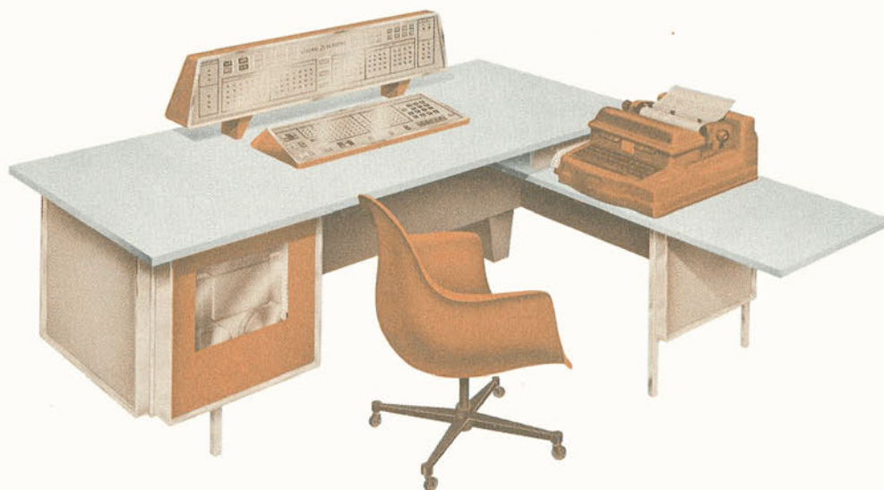
CONTROL CONSOLE, INCLUDING PAPER TAPE PHOTOREADER (LEFT) AND CONSOLE TYPEWRITER (RIGHT)
