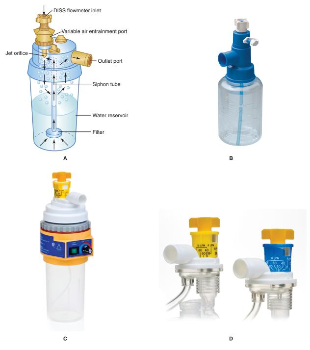
FIGURE 4-4 Large volume jet nebulizer: A. Schematic. B. Dry disposable. C. Heated disposable. D. Prefilled heated disposable. Photo B reproduced with permission from CareFusion. Photo C courtesy of Teleflex. Photo D coutesy of Teleflex.
