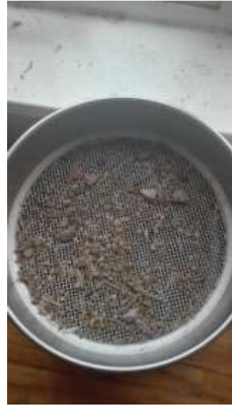
Larger gravel fragments have to be removed manually
