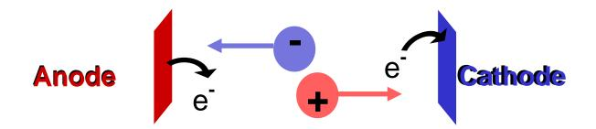
We are going to measure the **mobility**, or rate of migration, of NaCl ions in a water filled tray. Mobility,  $\mu$ , of a charged ion is described by
