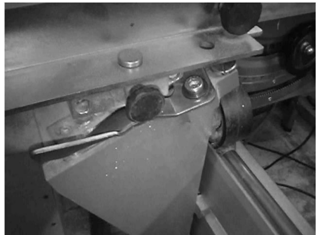
Figure 7: Lever for the guiding and fixation of the carriage.
