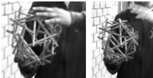
Figure 2: Tensegrity system built with cables, subjected to a perturbation; it doesn't change its shape.
