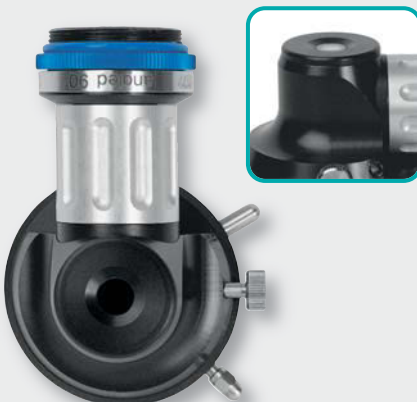
250-020-025 F=25mm (splitting 90/10) 250-020-030 F=30mm (splitting 90/10) Beamsplitter, allows simultaneous video and direct views, c-mount, soakable, Full HD
