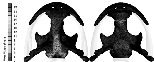
FIG. 3. Von Mises stress distribution in the skull of Chinese giant salamander (Marcé-Nogué et al. 2011)
