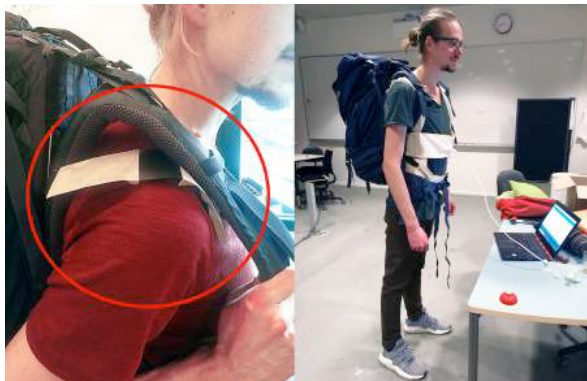
Figure 1: Positioning of the soft pressure sensors (left) and data collection set up (right)
