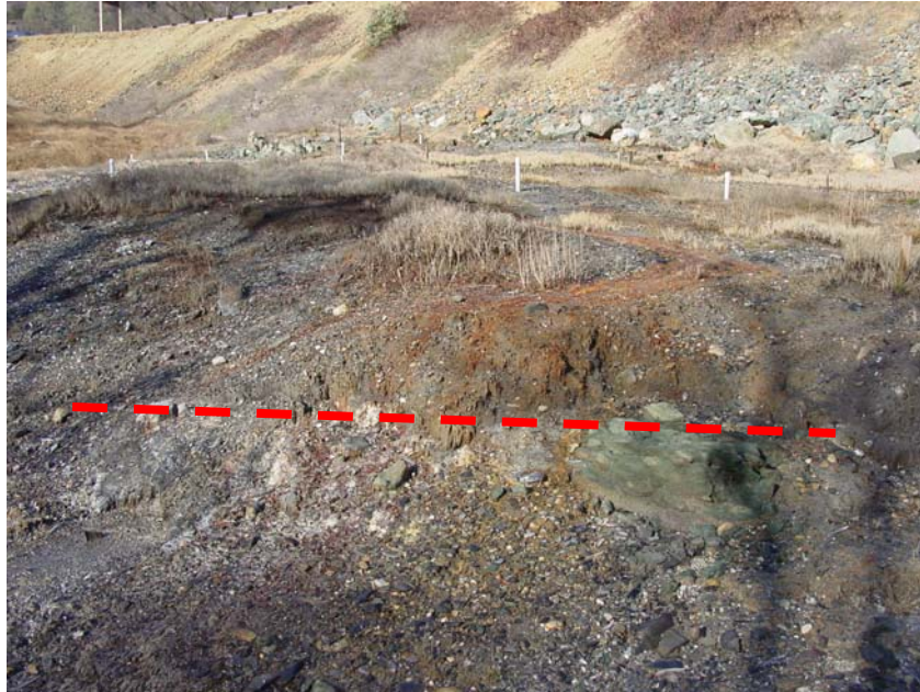
Figure 13 Fill thickness in Spring 2. Sediment above the dotted red line is fill.
