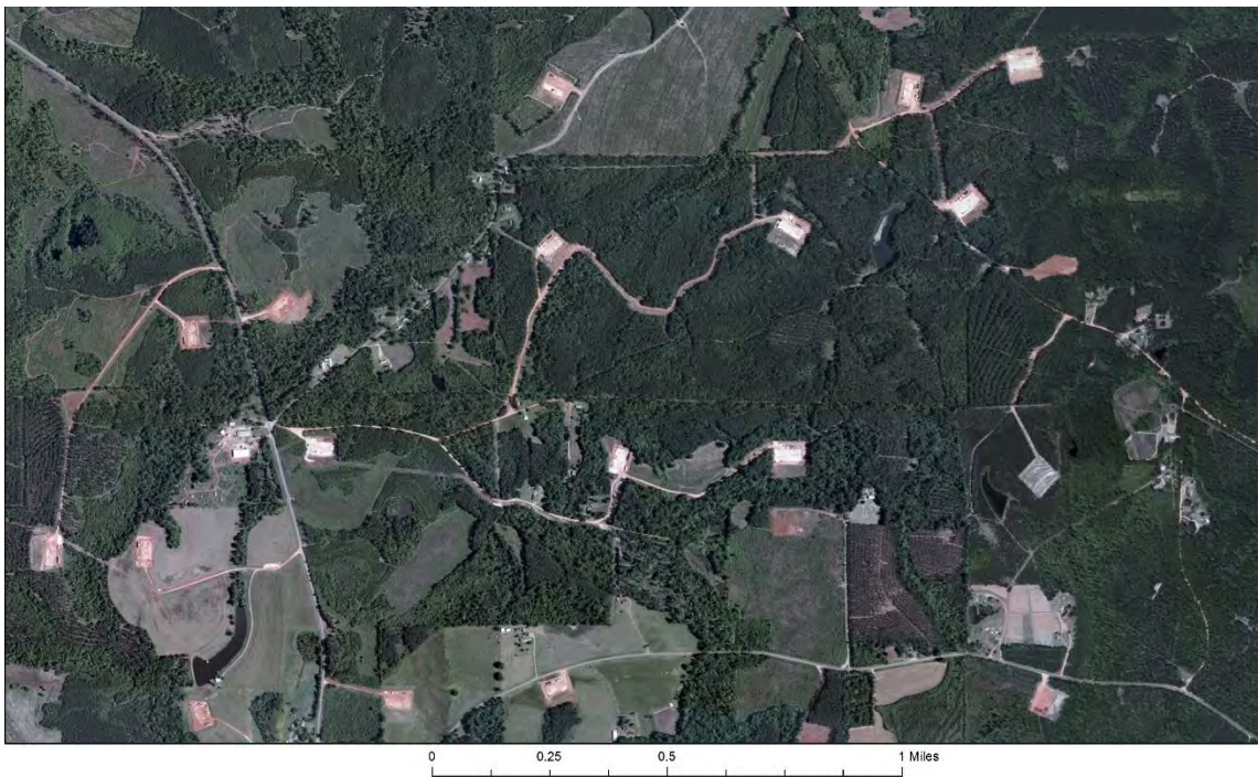
Figure 3-7. New well pads and access roads in a rural landscape, Conecuh County.
