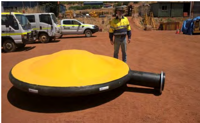
Plate 2.3: Example of a Turret Decant System
