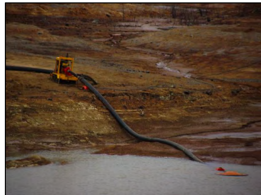
Plate 2.3: Example of a Turret Decant System
