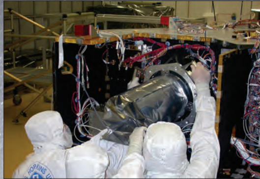
LORRI, a long-range reconnaissance imager, is a 1000 × 1000-pixel sensor that, in combination with a telescopic camera, delivers monochrome images and high-resolution geological data. LORRI measured Pluto's diameter at 1473 miles (2370 km).
