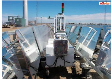
**Figure 23: eSolar's automatic cleaning robot (Source: eSolar).**
