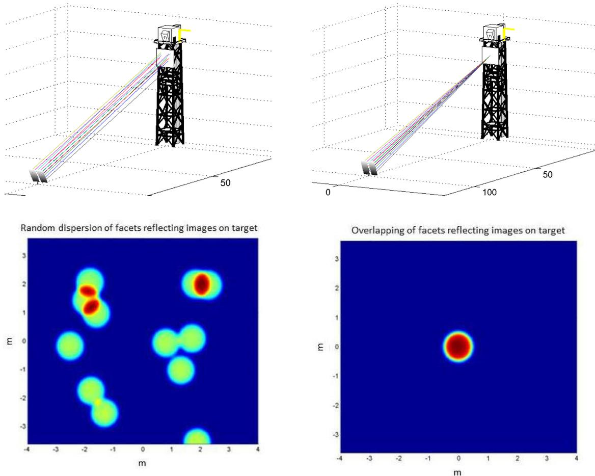
**Figure 12: Simulation of heliostat image on target before (left) and after (right) canting (Source: [Monterreal2014]).**
