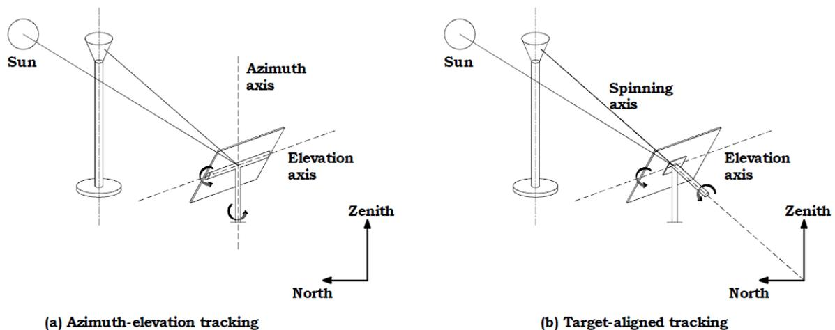
**Figure 13: Schematic representation of the rotations in two heliostat tracking modes: (a) azimuth-elevation tracking and (b) target-aligned tracking.**
