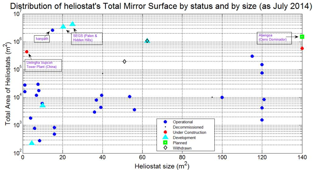
**Figure 17. Distribution of total Heliostat mirror surface deployed worldwide by project status and heliostat size.**
