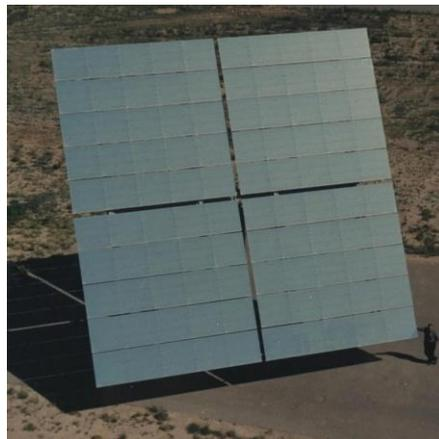
**Figure 19: Advanced Thermal Systems H150 heliostat on test at Sandia's NSTTF (Source: [Mancini2000]).**
