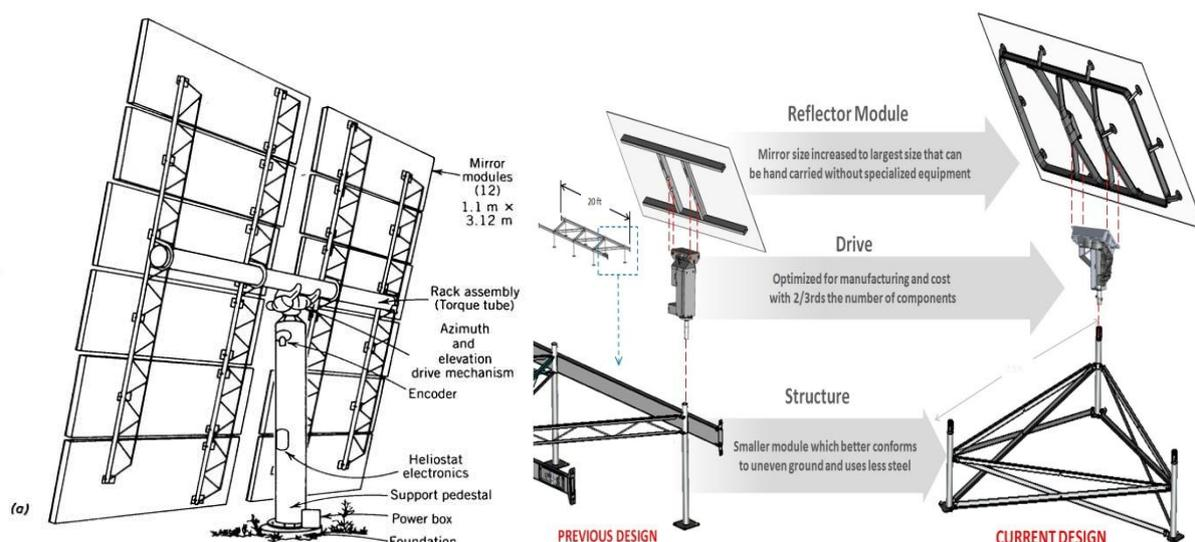
**Figure 2: Examples of typical elements in large (left) and small (right) size heliostats (Source: Left: Southern California Edison Co. / Right: eSolar).**
