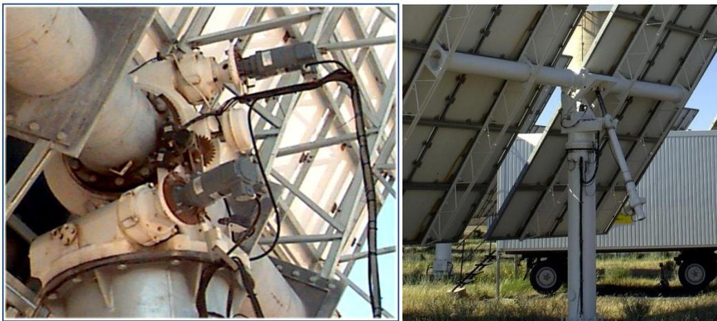
**Figure 9. Rotating and linear actuators based on rotary electromagnetic motors as power sources.**
