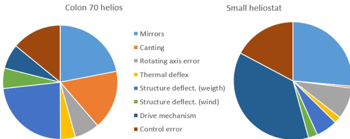
**Figure 22: Balanced “error budgets” for different heliostat configurations.**
