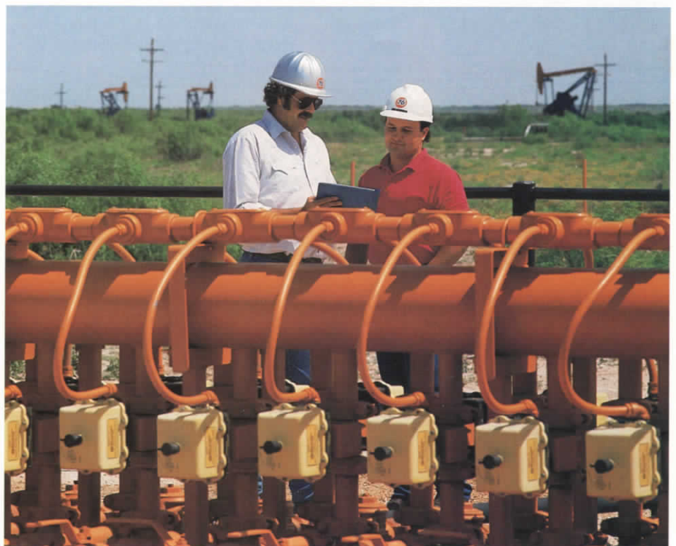
Above right, the Cerveza platform, Gulf of Mexico. Right, CO 2 injection in the Dollarhide field, West Texas. "The U.S. Gulf Coast, both onshore and offshore, will continue to be a very active area for Unocal," says John Imle.
