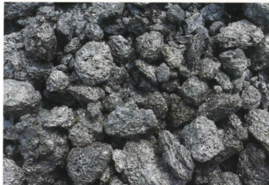
Premium needle coke produced by Unocal is used to make ultra high power electrodes.
