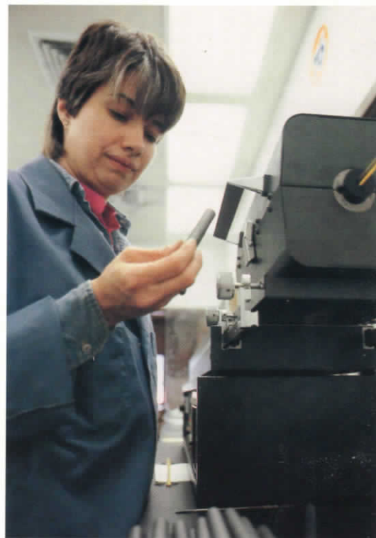
In the Chicago carbon plant's quality control lab, Mary Kay Miko prepares to test the CTE of a graphite rod made from needle coke.
