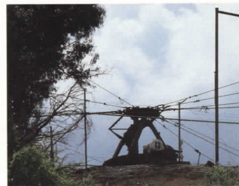
The sprawling Southern California District employs several different “vintages” of technology—from central-power driven jack lines on century-old wells (above) to the latest in offshore production techniques on Platform Gilda (right).
