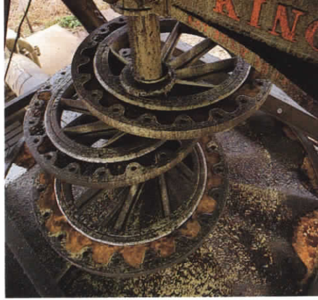
Clockwise from below: Brea's Imperial golf course, built over a district oil field; detail of a still-functioning 100-year-old jack line apparatus in the Bardsdale field near Santa Paula; pump jacks nod away at the nearby Torrey Canyon field.
