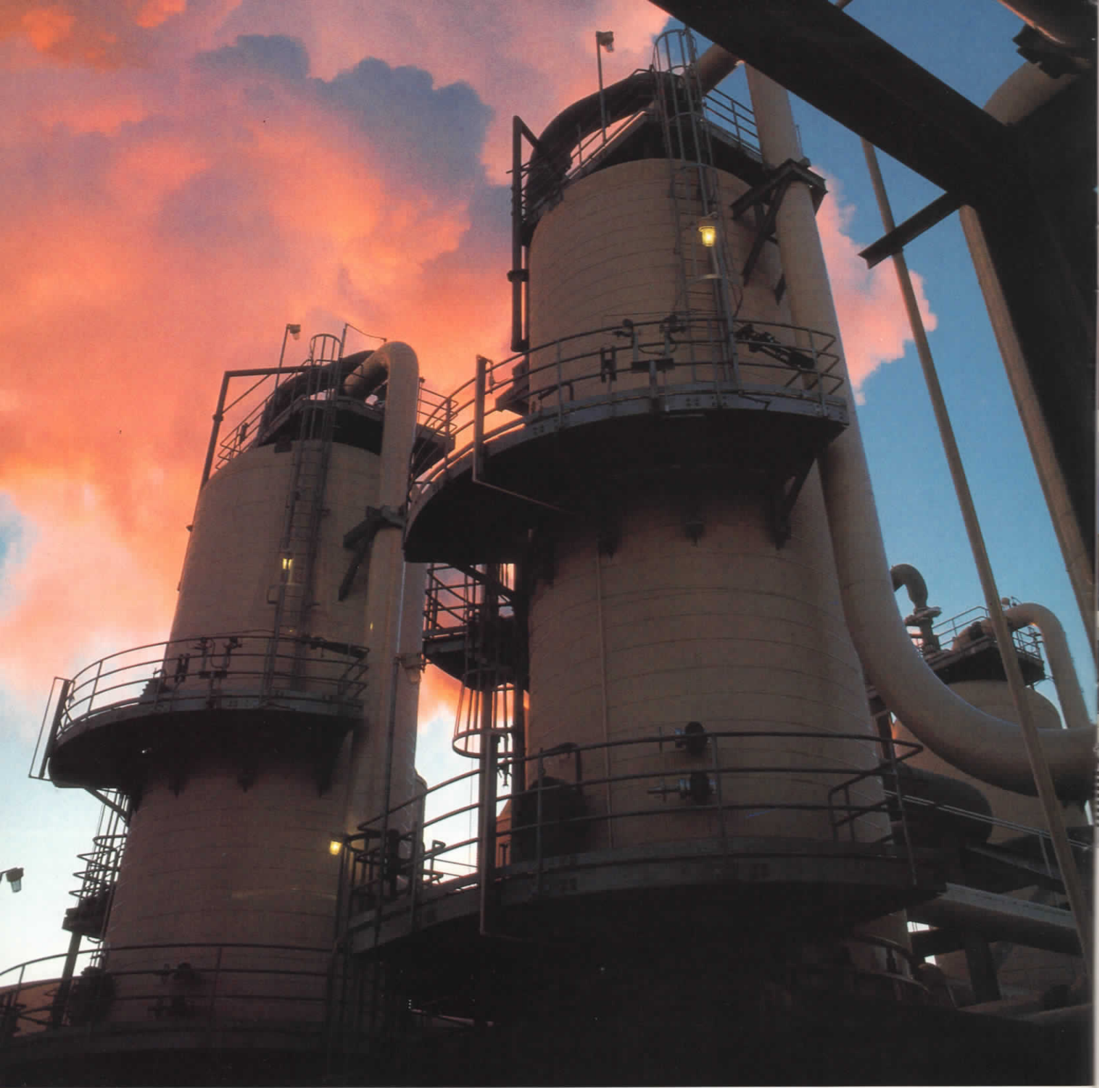
Above, Unit 3's standard and low-pressure crystallizers. Right, some of the 300 people who attended the facility's dedication ceremony.
