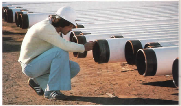
Above, corrosion specialist Mark Schilling inspects the protective coating on pipes that will be used for offshore production. Below, he studies the coating inside a crude oil storage tank. Left, test panels used to evaluate coatings for offshore equipment.
