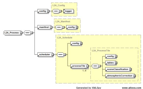
Figure 3-2 - High Level Processor Architecture
