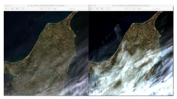
Figure 3-11 – Cirrus Correction over north Denmark, Bands 2-4 with Band 10. Left: L2A Output cirrus corrected, right: without correction.
