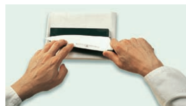
(d) Draw the knife across the stone all the way to the heel of the blade.
