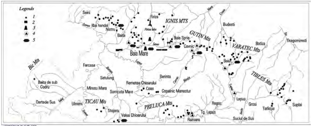
Fig. 1. Baia Mare ore district. 1. The main tailings; 2. Dumps; 3. Furnaces and chemical plants; 4. Old metallurgical objects; 5. Flotations.
