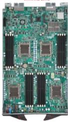
Tylersburg/Nehalem Storage Blade w/ 6 SAS2.0 HDD Support and QDR InfiniBand
