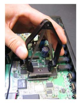
9. Once the EPROM is correctly aligned, use two fingers to press it home with gentle, even pressure applied to all of the pins at the same time. Once again, this does not require undue effort. Do not use force. If you feel resistance, stop immediately. Please keep an eye on all of the EPROM's pins—it's very easy to bend or even break them off, which would amount to the destruction of the EPROM.
