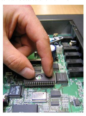
10. Finished? Then things should look exactly like this. Please note how the notch of the EPROM matches that of the socket.
