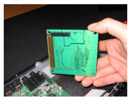
12. Next, place the board with the socket on the mating double row of contact pins. Be sure that the pins and sockets are aligned before pressing the board home.
