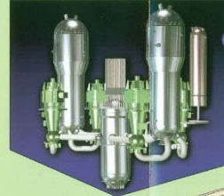
REACTOR COOLANT SYSTEM
