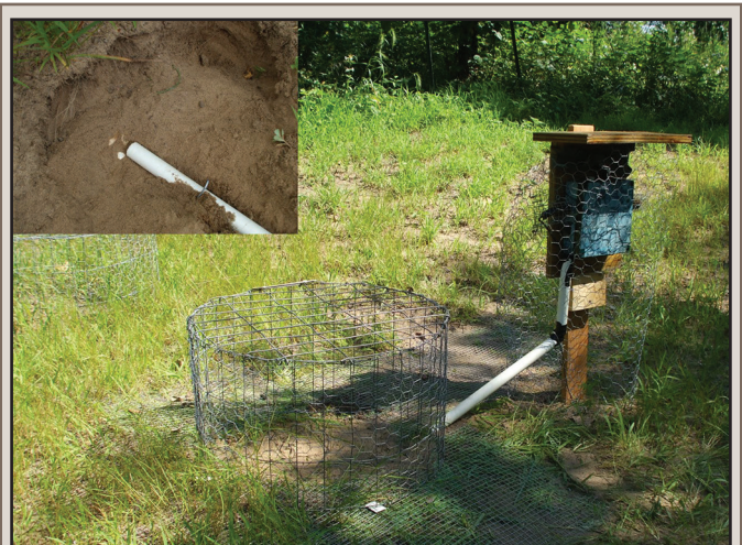
FIG. 1. Field equipment set-up used to acoustically monitor natural Graptemys ouachitensis nests. The main photo shows the acoustic monitoring unit and ambient microphone within chicken wire screening to prevent disturbance by raccoons ( Procyon lotor ) and the PVC pipe shielding the cabled microphone monitoring the cage-protected nest. The inset shows the PVC pipe housing the recording microphone near its open end, close to the clutch.
