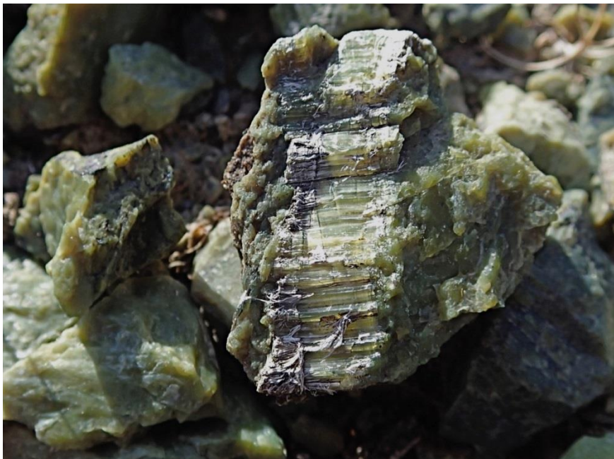
Figure 3. Fibrous chrysotile vein, 15mm wide, in serpentine.
