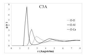
FIG. 1. RDF for cation-anion and anion-anion for binary system calcia-alumina (C3A).
