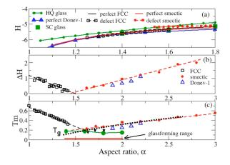
FIG. 1. (a) Crystal enthalpies H for perfect crystals FCT, Smectic B and Donev-1 at T = 0.1, compared with Hof glasses (SlowCooled and HyperQuenched) and defect crystals obtained from freezing liquids at aspect ratios  $\alpha =$ 1.1, 3.0, and 2.2, respectively, and then tuning  $\alpha$  within the crystal state (b) enthalpies of fusion (c)  $T_m$  and  $T_g$
