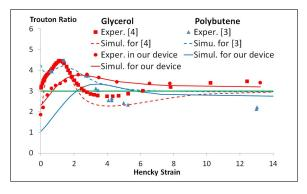
FIG. 1. Dependence of Trouton ratio on Hencky Strain for Newtonian liquids: squares - experimental data [4] for glycerol, triangles - experimental data [3] for polybutene. The dashed lines represent our simulations for corresponding liquids in CaBER-like devices [3, 4]. Circles - experimental data for glycerol in our device. The solid lines represent the simulations for our device.
