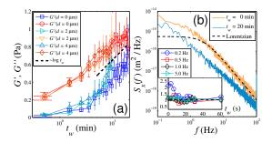
FIG. 1. (a) Time evolution of the storage and loss moduli (f = 5 Hz) after the quench in differents places inside the droplet (b) Power spectral density of fluctuations of x at two different  $t_w$ . Inset: Time evolution of the ratio  $\pi f S_x(f)/(2k_BTIm\{\chi(f)\})$  at different frequencies.
