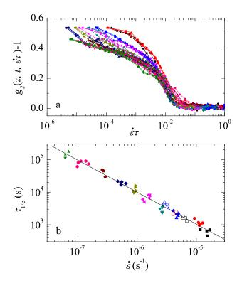
FIG. 1. a-The final relaxation ICFs collapses when plotted as a function of a rescaled time,  $\dot{\epsilon}\tau$  showing that the microscopic gel dynamics is directly related to its macroscopic deformation. b-Double logarithmic plot of the relaxation time  $\tau_{1/e}$  of the ICFs shown in a) as a function of  $\dot{\epsilon}$ .
