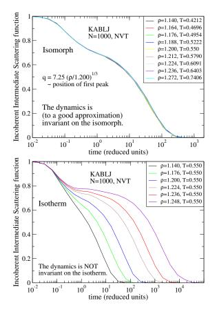
FIG. 1. Upper panel: Invariance of the inchoherent intermediate scattering function on an isomorph. State points on isomorph chosen to keep  $S^{ex}$  constant. Lower panel: Corresponing isotherm with slightly less density change.
