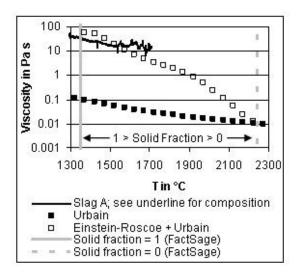
FIG. 1. Comparison of measured, normal calculated and solid-liquid calculated viscosities. Slag composition is  $Al_2O_3 = 1.0$ ; CaO = 39.2;  $Fe_2O_3 = 11.8$ ;  $K_2O = 1.6$ ; MgO = 23.1;  $Na_2O = 5.0$ ;  $SO_3 = 16.8$  (values in mass-%, trace amounts were neglected).
