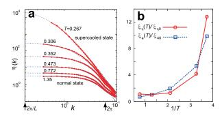
FIG. 1. (a) The k-dependence of  $\eta$  for several temperatures.  $\eta(k)$  can be well fitted by the empirical function,  $\eta(k=0,T)/(1+(\xi_{\eta}(T)k)^2+(\lambda_{\eta}(T)k)^4)$  (dashed curves), where  $\eta(k=0,T)$  is the macroscopic shear viscosity obtained by the Green-Kubo formula. (b)  $\xi_{\eta}$  and  $\xi_4$  scaled by their values at T = 1.15 are plotted against 1/T.
