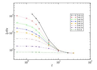
FIG. 1. Friction coefficient  $\xi$  of A particles in the binary Yukawa mixture at different temperatures as a function of the external force f.
