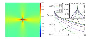
FIG. 2. Left:  $C(\vec{r})$  over  $\Delta \gamma = 1\%$  at  $\dot{\gamma} = 1e-05$ , T = 0.025and  $L \times L = 160 \times 160$ . Right:  $C(\vec{r})$  along the perpendicular direction of applied shear, for all strain rates. We zoom in the tail of  $C(\vec{r})$ . Arrow indicates increasing of  $\dot{\gamma}$ .
