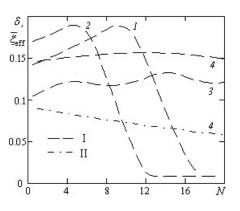
FIG. 2. Dependences of  $\delta$  (I) and  $\bar{\xi}_{\text{eff}} = 0.015\xi_{\text{eff}}$  (II) on N for linear viscoplastic (1, 2), elastic viscoplastic (3) and nonlinear viscous (4) fluids ( $\chi \to \infty$ , b = 1, c = 1): 1 –  $A = 0.2, \xi_0 = 12$  (Bn = 0.2); 2 – 0.2, 12 (Bn = 0.4); 3 – 0.1, 10 (We = 1, Bn = 0.5); 4 – 0.15, 7 (m = 0.75)
