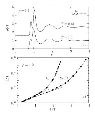
FIG. 1. Comparison between the LJ and its WCA description at the liquid density  $\rho = 1.2$ . Top: Static pair correlation functions. Bottom: Arrhenius plot of the relaxation time.
