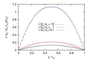
FIG. 1. Poiseuille flow of a non-linear Maxwell fluid.  $c_* = 0.1$  and  $G_{\infty}$  is set to 1 Pa. A pressure gradient  $\Delta p/L_x = -2$  Pa/cm with  $L_x = L_y = 1$  cm is applied.
