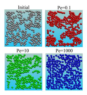
FIG. 2. BD simulation image slice of particle positions at steady states both at rest and under shear of a strong gel with  $\phi$ =0.44, revealing different levels of heterogeneity.
