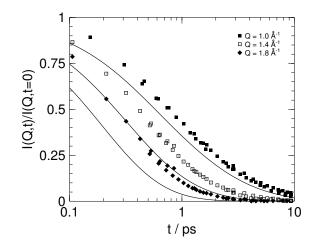
FIG. 1. Normalized incoherent intermediate scattering function for  $n-C_{100}H_{202}$  (symbols) and the Rouse prediction (solid lines) for three values of momentum transfer Q.
