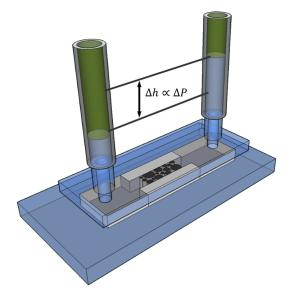
FIG. 1. A schematic of the experimental setup. The applied pressure is adjusted by the height of the two water columns connected to the porous structure.
