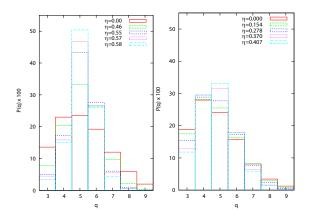
FIG. 1. The spindle order q (defect) distribution in bidisperse 3D (left) and monodisperse 4D (right) hard spheres shows a growing structural order as the volume fraction  $\eta$ of the fluid increases [9].
