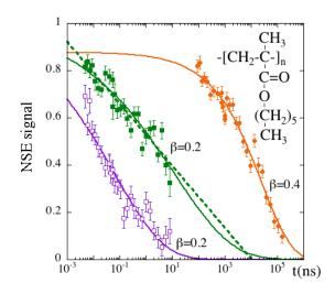
FIG. 1. Neutron Spin Echo signal measured on poly(hexyl methacrylate) probing the structural relaxation of MCs (full circles) and within the nanodomains (full squares), and the self-motions of SG-hydrogens (empty squares) at  $T \approx 320$  K (full circles have been measured at 480 K and shifted). Solid lines: fits to stretched exponentials  $A \exp[-(t/\tau)^{\beta}]$ ; dotted line: logarithmic description.
