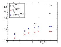
FIG. 1. Critical temperature  $T_c$  as a function of the endto-end radius  $R_{ee}^c$  (measured at  $T_c^{\rm MD}$ ). The theoretical values  $T_c^{\rm MCT}$  are compared with the simulation values  $T_c^{\rm MD}$
