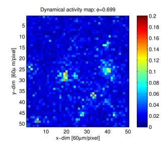
FIG. 1. Dynamical activity map constructed with the intensity structure function  $d_2(\tau = 1s, \mathbf{r})$  for a sample at  $\phi = 0.699$ .
