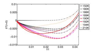
FIG. 2. Change in temperature,  $\delta T$  at the center of a sphere after a temperature step of  $\Delta T = 1$  has been applied at the surface (radius r = 10mm and parameters determined by Glycerol data). Time is scaled with the characteristic heat diffusion time  $\tau = \frac{r^2}{D} - D$  being the heat diffusion constant. The maximum occurs just above  $T_g$  (around 186K in Glycerol) where both shearmodulus and isobaric expansion coefficient are expected to be large.
