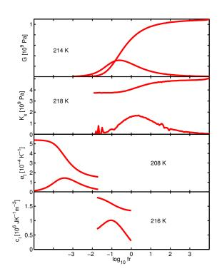
FIG. 2. Examples of the frequency-dependent data, from top: shear modulus  $G(\omega)$ , adiabatic bulk modulus  $K_s(\omega)$ , longitudinal expansion coefficient,  $\alpha_l(\omega)$  and the longitudinal heat capacity  $c_l(\omega)$ . Imaginary parts of  $K_s(\omega)$  and  $c_l(\omega)$  have been multiplied by a factor of 5.
