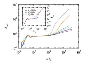
FIG. 2. Reduced creep compliance  $J_{red}$  for a polydisperse suspension at  $\phi_{eff} = 0.65$  vs. the reduced time  $t/\tau_0$ . The creep was performed at reduced shear stresses: 0.563 (grey), 0.469 (orange), 0.413 (green), 0.375 (light blue), 0.375 (red), 0.357 (dark blue) and 0.282 (black). This measurements were performed after a pre-shear and a waiting time  $t_w = 600s$ . The inset shows the waiting time dependency at a reduced shear stress of 0.912.
