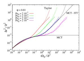
FIG. 3. MCT-ITT fits to mean squared displacements (solid in flow direction, dashed perpendicular to flow) of the system in Fig. 1 under shear and for a glassy state. The dimensionless Peclet number  $\text{Pe}_0 = \dot{\gamma}\bar{\sigma}^2/D_0$  compares the shear rate to the dilute Brownian diffusion time.
