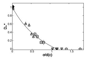
FIG. 1. Evolution of diffusion coefficient of colloidal tracers in Laponite normalized by the value measured in pure water,  $D_{\infty}^* = D_{\infty}(c)/D_0$ , as a function of the concentration of laponite for various tracer sizes: ( $\diamond$ ) 1 nm fluorescein molecules; ( $\triangle$ ) 25 nm diameter colloids; ( $\Box$ ) 37 nm diameter colloids;( $\diamond$ ) 100 nm diameter colloids.
