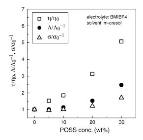
FIG. 1. Relative changes in conductivity (ion mobility) and viscosity, in relation to amount of 2 nm POSS molecules added to solvent cresol.
