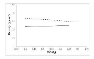
FIG. 2. Comparison of calculated (full line) and experimental (dash line) density of  $(CaO)_{1-x} - (SiO_2)_x$  mixtures at 2000 K.
