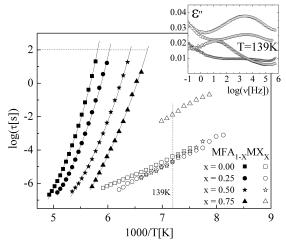
FIG. 1. Relaxation map for  $\alpha$ - and  $\beta$ - relaxation times (filled and open symbols respectively) in binary mixtures of m-FA and m-X. Inset shows a comparison of dielectric losses for different mixtures at T=139 K in the glassy state.
