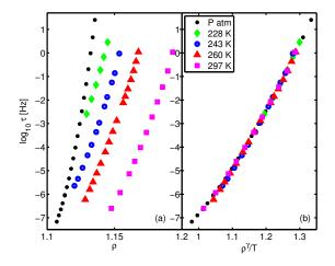
FIG. 1. Relaxation time ( $\tau = 1/\omega_{max}$ ) as a function of (a) density and (b)  $\rho^{\gamma}/T$  for DC704.  $\gamma = 6.1$
