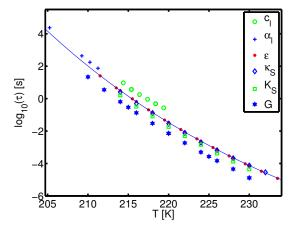
FIG. 1. Characteristic time scales (defined from loss-peak positions) as function of temperature for the six response functions of Tetramethyltetraphenyltrisiloxane (DC704). The line is a fit of the dielectric data to an Avramov function  $(\tau(T) = \tau_0 \exp{(B/T^n)})$ , used for extrapolation of the dielectric data to low temperatures.
