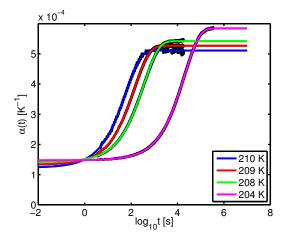
FIG. 2. Time dependent linear thermal expansion coefficient of Tetramethyltetraphenyltrisiloxane (DC704). The black lines are data and the colored lines are fits.
