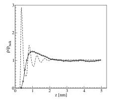
FIG. 1. Layering effect in the monomer density (dashed line) and chain center-of-mass density (circles) of a confined 1,4-polybutadiene melt. Both curves are normalized by the corresponding density in the bulk [4].
