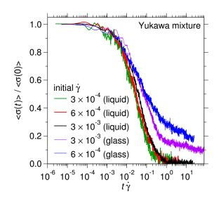
FIG. 1. Shear stress  $\langle \sigma(t) \rangle / \langle \sigma(0) \rangle$  as a function of  $t\dot{\gamma}$  after switching off shear in the steady state of a binary Yukawa mixture at the indicated shear rate  $\dot{\gamma}$ . The liquid and the glass state correspond to the temperatures T = 0.14 and T = 0.05, respectively [2].
