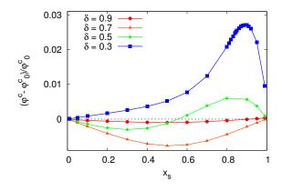
FIG. 2. Glass transition lines for different radius ratios  $\delta$  as a function of the concentration of small particles  $x_s$ . The glass is stabilized for small radius ratios while the liquid is stabilized for large radius ratios.
