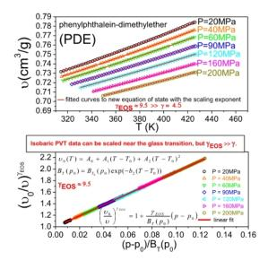
FIG. 1. The upper panel shows a succesful fit of PVT data for PDE to a non-configurational isobaric counterpart of Eq. (2). The scaling of the specific volume in terms of this equation is presented in the lower panel.
