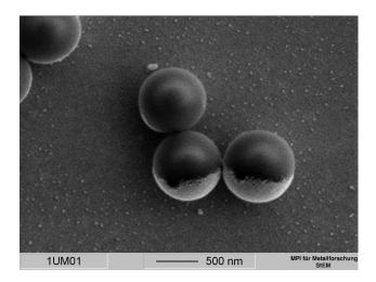
FIG. 1. Janus particles. SEM image of  $1 \,\mu$ m diameter silica particles half-coated with a 50 nm layer of gold (lighter color).
