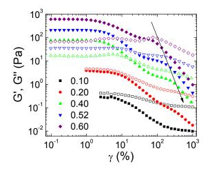
FIG. 1. Dynamic strain sweeps of different volume fractions with equal attraction strength of Udep(2R)=-19kT. Note the complicated behaviour of G' (solid) with increasing strain and the dissipation of the second G'' (open) yielding peak (100% strain) with decreasing volume fraction. The arrow shows the approximate shift of the second G'' peak with decreasing volume fraction.
