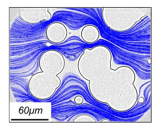
FIG. 2. Trajectories of colloidal particles flowing through a random porous structure.
