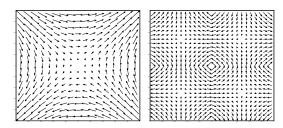
FIG. 1. Velocity field of (left) a simple extensional flow and (right) a smart periodic continuation of an extensional flow used as a simple model to study gravity-driven convection.
