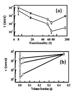
FIG. 1. (a)  $\tau$  vs f for polymer grafted nanoparticles and (b)  $\tau$  vs volume fraction,  $\phi$  for their binary mixtures. In (a) squares represent data collected at 100<sup>0</sup>C and uptriangle for data collected at 115 <sup>0</sup>C for q = 0.03 Å<sup>-1</sup>. In panel (b) data is shown for 105 <sup>0</sup>C and same q as in (a).
