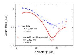
FIG. 2. Polydisperse RDG-Fit to conventional and by TCDLS corrected data. The fit is only in good agreement with the MS-free data. While both fits determine the particle size correctly, the SLS data leads to unreasonable high polydispersities.
