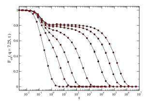
FIG. 2. The incoherent intermediate scattering function at  $\rho = 1.2$  and T = 2.0, 0.80, 0.60, 0.50, 0.44, 0.42 and 0.405 (left to right) for the *KA* binary mixture. The *NVE* dynamics is given by filled black circles and the *NVU* dynamics as red crosses.
