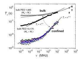
FIG. 2.  $T_1(\omega)$  as measured by FCNMR [2] of bulk PEO (upper curves) and confined in SMM (lower curves) for pore diameters of 8nm, 13nm, 21nm, 33nm and 58nm at 358K.
