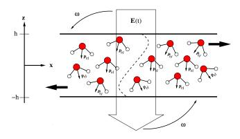
FIG. 1. Illustration of flow generation using a rotating electrical field,  $\mathbf{E}(t)$ . The water molecules have a permanent electrical dipole, here denoted  $\mathbf{p}_{el}$  which is not perfectly aligned with the field due to thermal fluctuations. The velocity profile is indicated by the dotted line and illustrates the opposite flow directions as shown by the thick black arrows.
