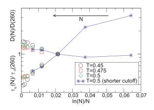
FIG. 1. The size-dependence (N = 65, 130, 260, ..., 8320) of the diffusion constant D (open symbols) and the structural relaxation time  $\tau_{\alpha}$  (filled symbols) in relation to its value for N = 260. Whereas the diffusion constant only displays very minor finite size effects, dramatic effects are observed for the structural relaxation time.
