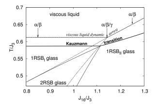
FIG. 1. Phase diagram of the 3 + 16 spherical spin model with dymanic (dashed) and thermodynamic (full) transition lines.
