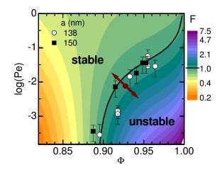
FIG. 1. Flow-stability of concentrated hard-sphere colloids versus reduced concentration  $\Phi$ . Symbols: experimental data of the reduced critical flow rate  $\text{Pe}_c$  below which shear banding occurs. Line: theoretical prediction for  $\text{Pe}_c(\Phi)$ based on Eq. (1). Colors show the value of F. The arrow shows a possible evolution of an unstable state.
