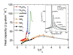
FIG. 1. Heat capacity of  $Fe_{50}Co_{50}$  through  $T_g$  compared to those for SiO<sub>2</sub> and BeF<sub>2</sub> as well as that for nanoconfined water. Filled symbols: experimental data. Open symbols: simulations. Inset: Heat capacity of argon in the vicinity of its liquid-gas critical point.(Taken from Ref. [1])
