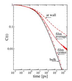
FIG. 3. Inhomogeneous relaxation functions for doublebond rotation dynamics in two different layers of confined polymer: In film center we obtain similar dynamics as in bulk, whereas at solid wall the relaxation is slowed down significantly, which also affects the average signal from the whole film (as it can be measured in NMR experiments).
