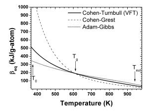
FIG. 1. Reduced free volume formation enthalpy in the equilibrium liquid,  $\beta_{eq}$ . The solid, dashed and dotted lines represent  $\beta_{eq}$  calculated according to each free volume model indicated in the legend. The temperatures shown are the VFT-temperature,  $T_0$ ; the glass transition temperature,  $T_g$ ; and the melting temperature,  $T_{eut}$ .
