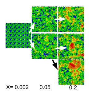
FIG. 2. Slab of the system for various values of the evolving crystallinity X. Particles are coloured according to the degree of crystalline order in their neighbourhood (blue,  $0 < Q_6 < 0.15$ ; green  $0.15 < Q_6 < 0.25$ ; yellow  $0.25 < Q_6 < 0.35$ ; orange  $0.35 < Q_6 < 0.45$ ; red  $0.45 < Q_6 < 0.55$ ). The initial state (left) has a periodic density pattern that is quickly forgotten.
