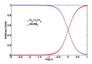
FIG. 1. Sketch of overlapping relaxations of  $G/M_T$  and  $(c_p - c_V)/c_p$ . The relative difference  $(c_p - c_l)/c_p$  depends on the product of the two relaxing functions. The higher a value at the inflection point, the bigger a difference between  $c_l$  and  $c_p$ .
