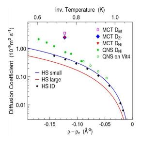
FIG. 1. Diffusion coefficients in binary Zr-Ni obtained from quasielastic neutron scattering (QNS) and calculated within MCT using partial S(q) is input. Results for a hard sphere (HS) mixture with equal particle size disparity is shown for comparison.
