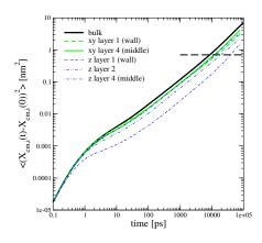
FIG. 2. Mean-square-displacement of the center-of-mass of chains in bulk and in different film layers, in directions parallel (xy) and perpendicular (z) to the solid wall [4].
