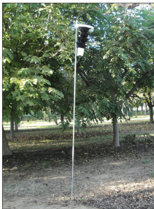
Figure 10. A four-unit funnel trap in place at the top of a pole.
