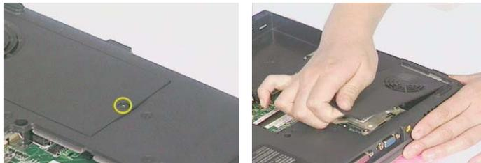
3. Remove the two screws that fasten the fan.
