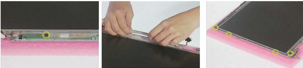
6. Remove the LCD from the LCD panel.
