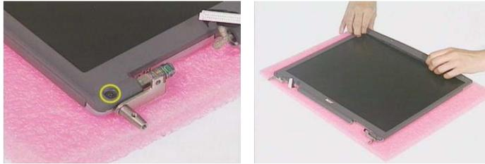
3. Unscrew the screw that holds the LCD inverter.
