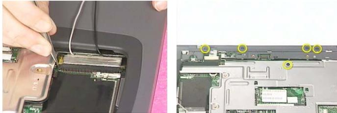
3. Remove the two screws as shown here.
