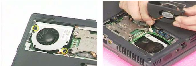
5. Remove the four screws as the picture shows.
