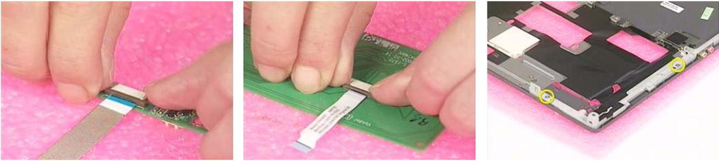
18. Unscrew the two screws that fasten the other hinge saddle.
