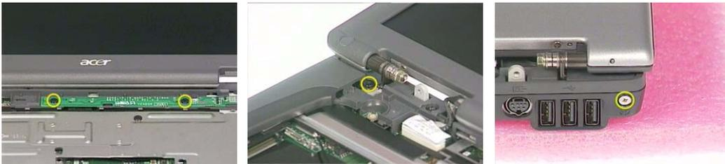
6. Take the two screws off the bottom panel as shown here, one on each side.
