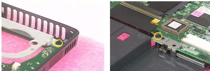
3. Remove the four hex head cap screws holding the main board.
