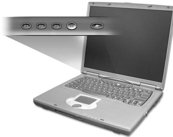
**NOTE:** To the left of these five launch keys is the wireless communication button. This wireless communication button works for model with 802.11b wireless LAN only.
