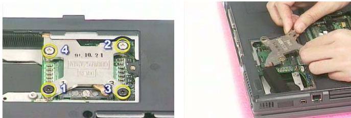
7. Unlock the CPU lock with the flat head screwdriver.
