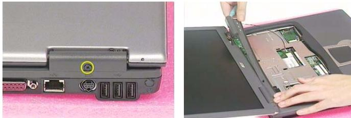
3. Remove the two screws holding the switch board.
