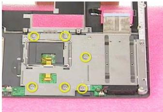
9. Tear off the mylar that fasten the touchpad FFC then disconnect the FFC.
