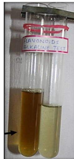
Fig. 4. Alkaline Reagent Test: Increased Intensity of Yellow Colour (Arrow) - Positive for flavanoids
