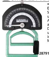
• 28791 SMEDLEY HAND DYNAMOMETER - aluminium Spring type hand dynamometer used to measure grip strength. Adjustable handle comfortably accommodates any hand size. Dial indicator remains at maximum until reset and is calibrated both in kg (0-100) and pounds (0-220). Manual in: GB, FR, IT, ES.
