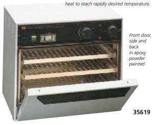
**TECHNICAL SPECIFICATIONS TAU 1.6** TAU 6 **TAU 18** 385x170xh 90 375x230xh 200 Inside dimensions (mm): 245x115xh 55 Outside dimensions (mm): 495x310xh 220 440x310xh 380 310x180xh 180 Weight: 5 kg 10.5 kg 14 kg Operating voltage: 220 V 220 V 110V available on request 250 W 600 W 400 W Power consumption: 3.15 A Fuses: Thermostat: Automatic capillary bulb type with self registration from 90° to 200° Timer: from 0 to 120 minutes high precision with capillary bulb Thermometer: Made in Italy
