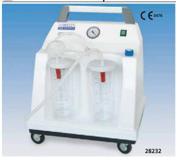
Ideal for hospital, these suction aspirators are manufactured in ABS. Four antistatic castors, two of which with brakes, to allow perfect mobility. Vacuum gauge for the control of vacuum (1 bar). 2 or 4 litre jar made of autoclavable makrolon, with 200/400 ml graduation. Each jar with double security valve. Pump piston type, lubrication and maintenance free. With anti bacterial filter. Available model with footswitch and other operating voltage (110 V).
