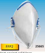
Facial filtering respirators to protect against solid (nonoil) and liquid (oil) volatile particles. With exhalation Valve (excluding 25665). Double elastic with buttonhole allows to hang the mask to the neck when it's not worn. Aluminium adjustable nose piece welded with high resistance and internal Polyethylene (PE) Foam nose pad. Single packed guarantees total hygiene and easy maintenance.
