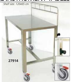
27914 INSTRUMENT TABLE 1 SHELF Operating room instruments table made of stainless steel AISI 304, scotch brite finish. Stainless steel adjustable 105-136 cm upper part with 4 instrument hooks. 125 mm Ø revolving castors (2 with brake). Weight: 21 kg. Load: 40 kg. Size: 120x65xh 95 cm. Delivered in kit form (123x13x68 cm).
