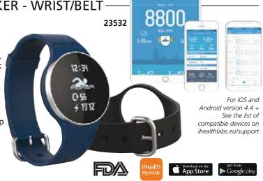
Battery: 1x3.7V Li-Ion 100 mAh - 3 years life. Supplied with 2 wrist bands (23532: blue and black) or 4 wrist bands (23531: black, grey, orange, pink) belt-clips (only 23531) batteries and USB cable for charging.
