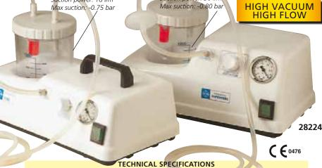
28222 Tobi 28224Super Tobi 220-230 V - 50/60 Hz 220-230 V - 50/60 Hz Operating voltage: 184 W 106 W Power consumption: 1,000 ml 1,000 ml Bottle capacity: 18 l/min 40 l/min Flow (air litres/min): -0.75 bar (563mm/Hg) -0.80 bar (600mm/Hg) Max suction: Working time: minutes 20 ON / 40 OFF 120 ON / 60 OFF Size (cm): 37x22xh 21 cm 37x22xh 21 cm Weight: 3.5 kg 5.25 kg IEC 601-1 IEC 601-1 Norms:
