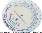
• 27336 BMI CALCULATOR - box of 10 Used in hospital and surgeries gives an indication of general health through the ratio of weight to height. Made of 2 rotating discs: 108 mm diameter (base) and 76 mm (top). Can be personalized with your logo for a minimum of 1,000 pieces.
