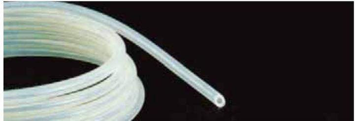
**SILICONE TUBES** for external medical use - silicone 100% Suitable for autoclaving (135°C - 2.2-2.5 bar) and Gamma Sterilization. Resistant to hot air up to 200°C. Infra-red vulcanization. Hours treatment at 200°C temperature in special oven. Anti-adherent, avoid incrustation and coagulation. Medical Grade - Transparent - Odourless
