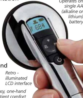
Operates on single AA (alkaline or lithium) battery
