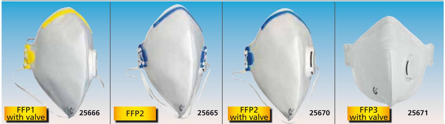
Facial filtering respirators to protect against solid (non-oil) and liquid (oil) volatile particles. With exhalation Valve (excluding 25665). Double elastic with buttonhole allows to hang the mask to the neck when it's not worn. Aluminium adjustable nose piece welded with high resistance and internal Polyethylene (PE) Foam nose pad. Single packed guarantees total hygiene and easy maintenance.
