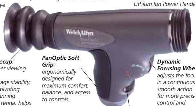
Patient Eyecup: allows proper viewing distance, provides image stability, serves as a pivoting point for panning around the retina, helps with orientation, and screens out ambient light. The eyecup is cleanable and reusable
