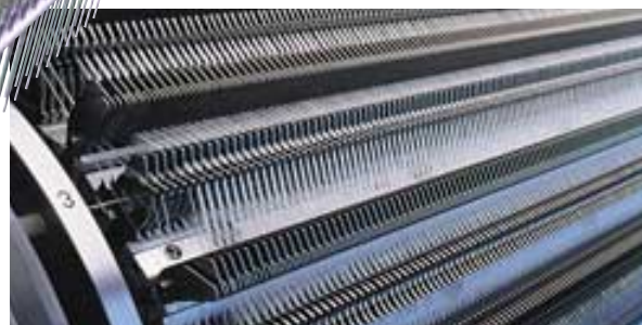
■ The wefts are inserted in staggered formation and guided to the fell by the movement of the rotor.
