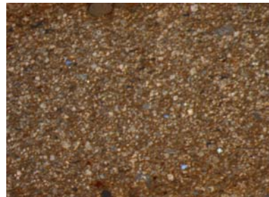
Well-sorted, fine-textured, higher rock content (clay matrix contains abundant discrete dolomitic grains) In houselots N25 & N11-28
