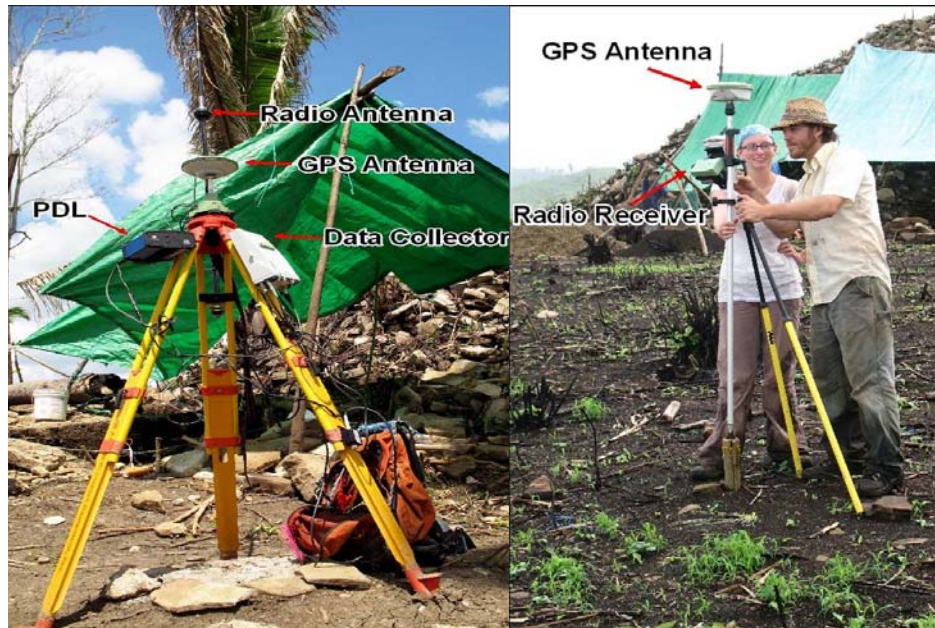
Figure 4a. Leica GPS System 1200 Base Station; (4b) Leica GPS System 1200 Rover
