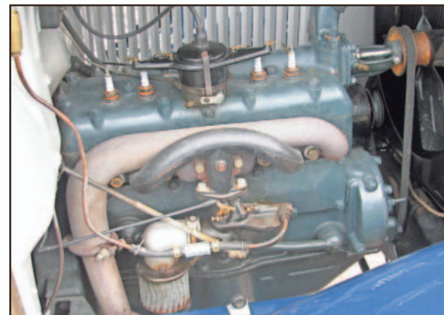
Original 4-cylinder engine except for upgraded carburetor air filter
