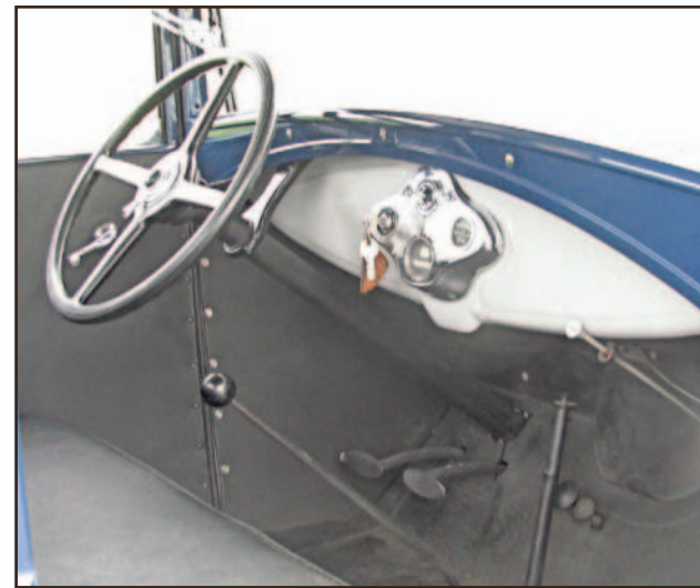
Meager dash, instrument cluster, floor shifter of 3-speed for manual transmission, emergency/parking brake lever and original heavy-duty steering wheel
