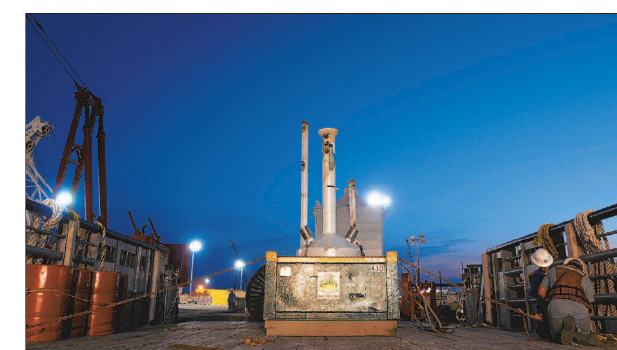
Associated Press A small pollution containment chamber, known as the "top hat," is loaded onto the deck of the motor vessel Gulf Protector on Monday in Port Fourchon, La. BP announced Wednesday that the "top hat" was on the sea floor near the wild well that has spewed at least 4 million gallons of oil into the Gulf of Mexico.
