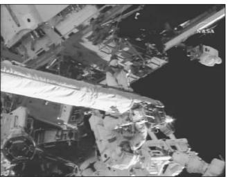
Astronaut Stephen Bowen adjusts a cable Wednesday on the end of the orbiter boom that was inhibiting a camera from maneuvering correctly.
