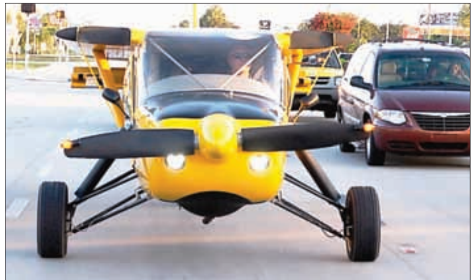
A Glasair Sportsman airplane mounted on the PlaneDriven package turns the plane into a street legal motortrike. The aircraft is at the end of the testing phase
