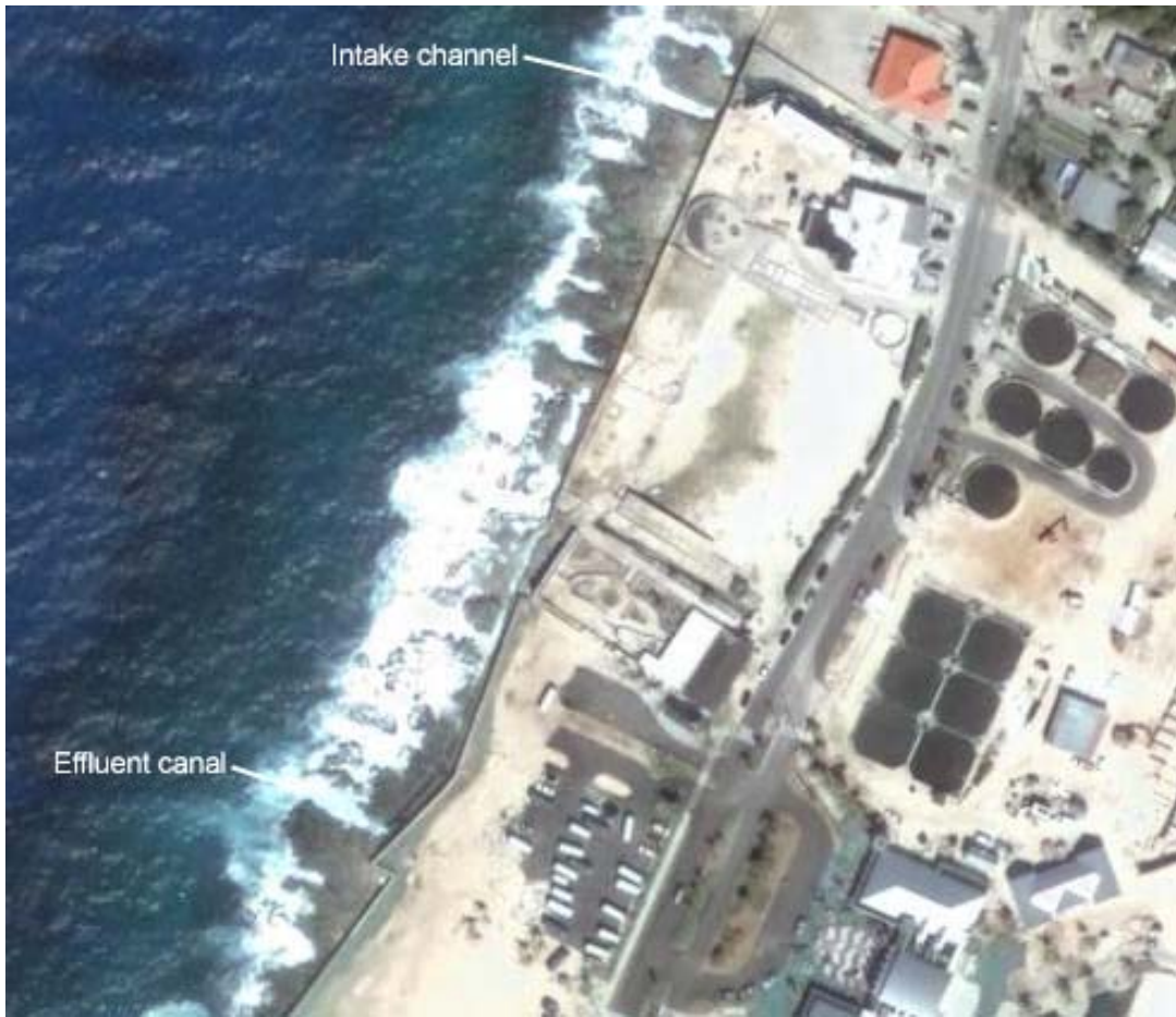
Figure 4-2. Satellite image of the Cayman Turtle Farm, Limited, Grand Cayman Island. The intake and effluent channels are labeled and are approximately 215 meters apart. The side-by-side round and square structures are tanks used for rearing C. mydas .
