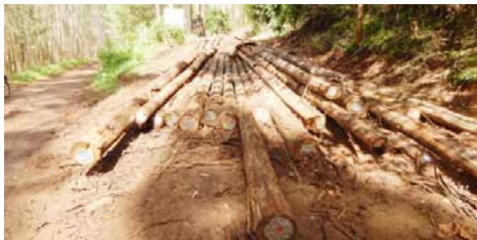
Transmission poles of 12m length, from seven-year-old trees.
