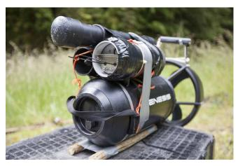
Figure 5. The C-Logger mounted on a Scooter
