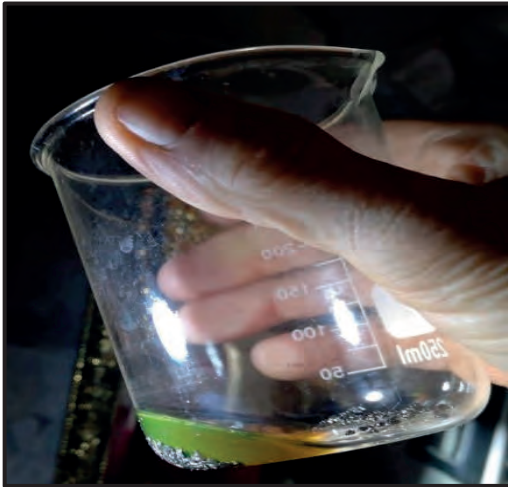
Figure 3: Demonstrates a strong positive trace after elution by shining a LED light in a dark room at right angles, four days after the tracer was introduced to Fluted Hole.
