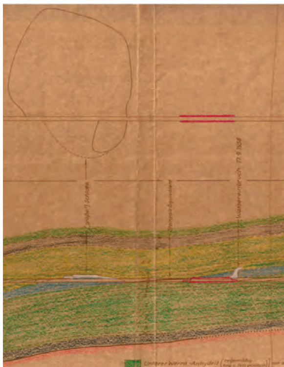
Figure 3: Section of Jung's profile showing the salt caves no. 10 (Big Schlotte) and no. 11 (Schlotte at water inrush from September, 17th 1958), compare with Fig. 4.
