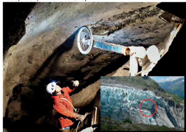
Figure 1: Lognan Ice Fall. Subglacial cavity and cavitometer, 2019, cl. L.M.
