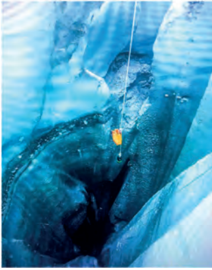
Figure 6: Lowering of the Leica BLK2GO dynamic scanner in the middle of the shaft and below with the adapted lighting (Méandre Technologie / Focale fixe), cl. M. Dalmasso
