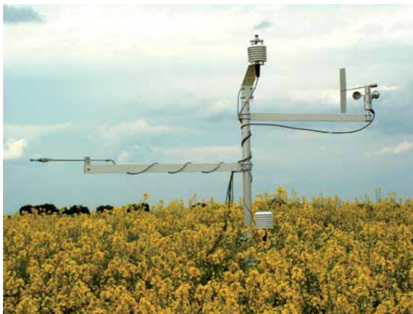
Fig. 1. BREB installation over winter rape-seed field: radiation balance gauge on left, pair of temperature/relative humidity sensor in the middle (upper with global radiance gauge), anemo-indicator on right. Locality: Červený Újezd 2006, photo by authors.
