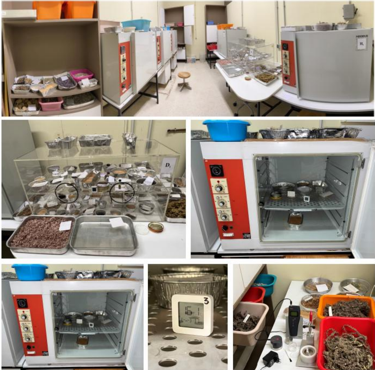
Figure 7. Seed drying. Above: A panoramic picture of the drying room kept at a quite constant temperature of 16-17 °C and a relative humidity between 40 and 50%. Middle row: The plexiglass drying chamber (left) and one of the 5 Heraeus chambers which served as germinators and have been currently reassigned as insulated drying chambers. With the help of desiccant (silica gel) the relative humidity in all 6 chambers is between 15 and 25%. Bottom right: A Rotronic HydroPalm portable instrument for highly accurate measurements of the equilibrated relative humidity over seed samples; these measurements provide relatively accurate estimates of the water content of a seed sample and, as a result, help us decide when seeds are sufficiently dry to be transferred into air- and water-proof vessels for long term storage at -20 °C.
