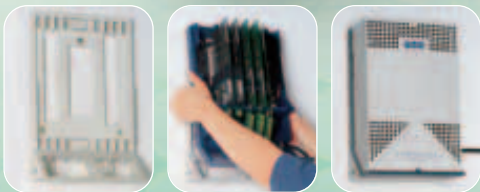
The mounting of the system is pretty easy: chassis on the wall, put on the rack, equip with modules, cover on, finished.
