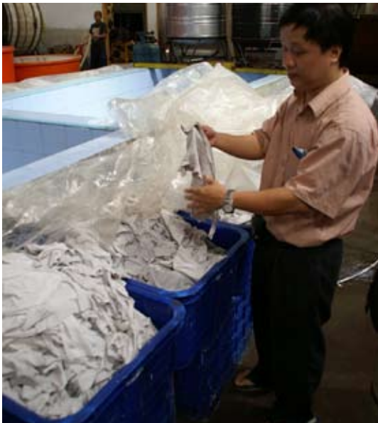
Monitor skins are bleached before they are stained and processed into high-quality leather products for western consumers. Skin factory, Macassar, SW Sulawesi, Indonesia. Photograph by André Koch .
