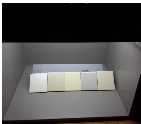
Figure 2 AMS standards Ceramic tiles which are used for the HVI calibration (Left to right: White, Brown, Yellow, Grey, Central)
