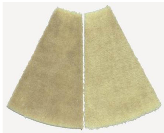
Figure 3 Carpets made from untreated yarn (left) and Lanasan NCF treated yarn (right) after Wools of New Zealand/International Wool Secretariat Rapid Soiling Test TM 267
