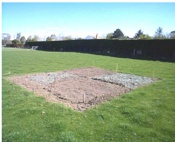
Figure 5 Trial plot immediately prior to seeding. Shredded carpet had been incorporated into the left and right quadrants, and a small amount of shredded carpet is visible on the surface of the soil
